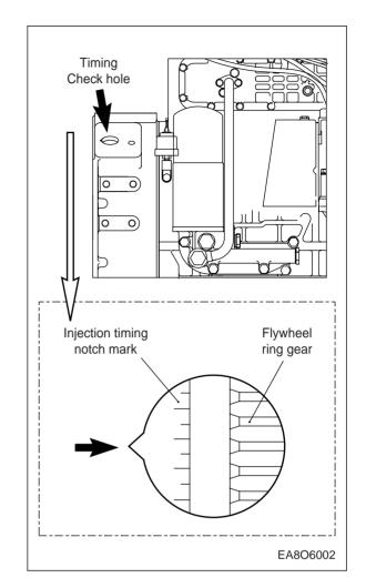
• Turn the timer until the notch mark of the indicator plate attached to the fuel injection pump is aligned with the notch mark of the timer.
