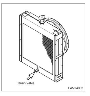
c) Loosen the coolant drain plug.
