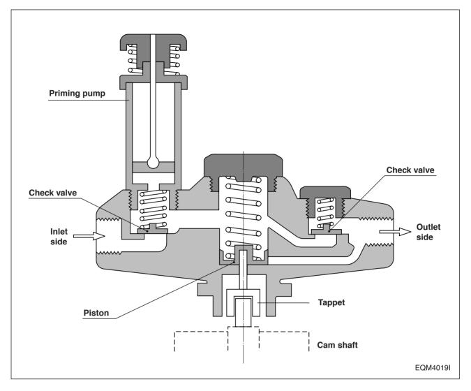
The P-type injection pump is mounted with K-ADS or KP type feed pump. These pumps have the same basic construction and operation, and the general descriptions of the KP type pump are given below:
