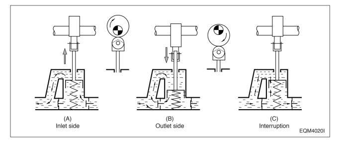
This feed pump is mounted with a priming pump designed to permit manual feeding of fuel from the fuel tank with the injection pump mounted in the engine. During the manual feeding operation, air must be bled from the fuel lines.
