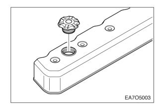
• Thereafter shut down the engine. After waiting for about 10 minutes measure the quantity of oil and refill the additional oil if necessary.
