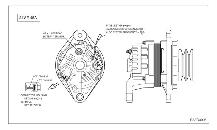
The alternator is maintenance-free, nevertheless, it must be protected against dust and, above all, against moisture and water.
