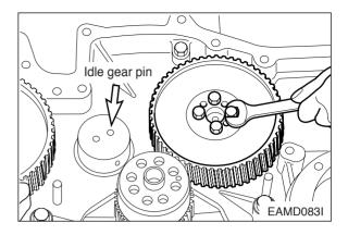
With the oil port on the idle gear pin facing the cylinder block, install the idle gear pin.
