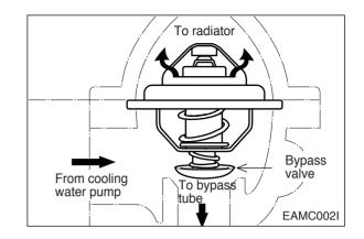
water passage to the radiator is opened so that the coolant is forced to flow into the radiator.
