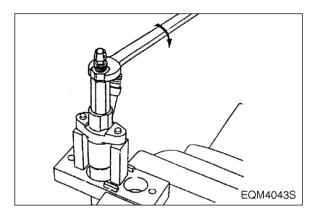
d. Install a nut (157892-1000 : SW 17mm) on the holder.
