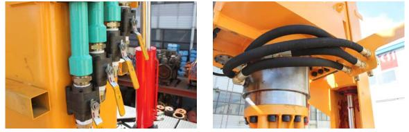
$1^{sT}$  PORT : Air Lifting  $2^{nd} \sim 4^{th}$  PORT : Cluster Hammer
