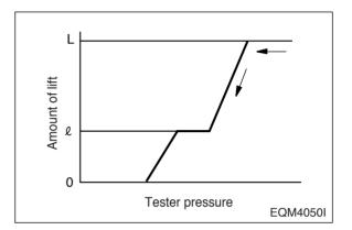
b. Take the indicated value on the dial gauge at the point of time when the secondary spring completes its operation and the needle valve puts an end to descent (the position of needle valve lift value "l" as shown in the above and right figures) and check that the value is within the specified limit.
