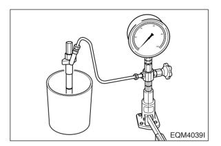
b. When replacing the nozzle, replace it with a new "nozzle service kit" integrated with a nozzle, lift piece, and spacer as a complete set.
