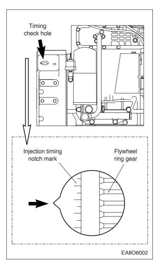
Turn the timer until the notch mark of the indicator plate attached to the fuel injection pump is aligned with the notch mark of the timer.
