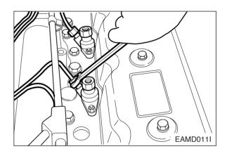
• Semi-assemble the nuts at both end of the fuel injection pipe and tighten them up one by one to specified torque.
