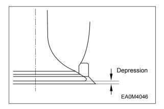
• For removal of the valve seat, apply arc welding work to two points of valve seat insert, and pull out the valve seat insert with inner extractor.
