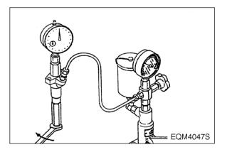
Operate the nozzle tester and increase the tester pressure up to 350 ~ 450kgf·cm<sup>2</sup> in order that the needle valve can be fully lifted. Then, record the full lift value "L".
