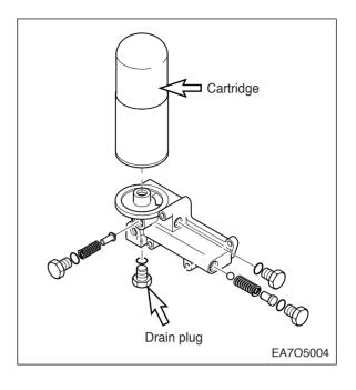
until sealing face is fitted against the O-ring. Turn 1-1/4 turns further with the filter wrench.
