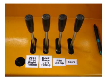
Deck Base Tilting : Right and left deck is opened and closed for drilling tool installation.
