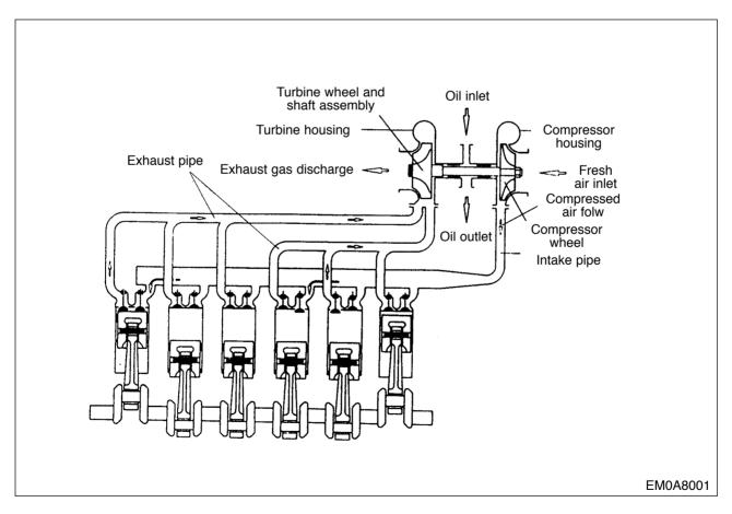
The turbocharger is a system designed to make use of the engine exhaust gas energy to charge high-density air into the cylinders, thereby to increase the engine output.
