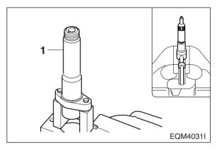
d. Assemble adjusting shim (10), secondary spring (11), and spring seat (12) on the nozzle holder body in the order as described.
