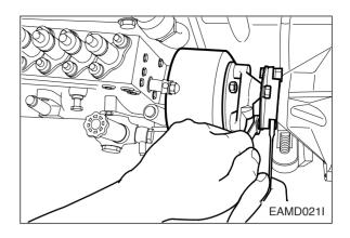
• Tighten the drive shaft connecting flange fixing bolts to specified torque.
