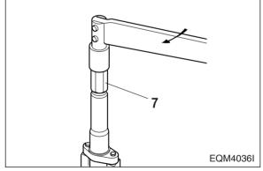
i. With the cap nut facing upward, install the nozzle holder on the plate.
