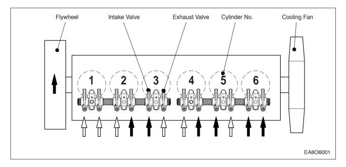
• No. 1 Cylinder is located at the side where flywheel was installed.
