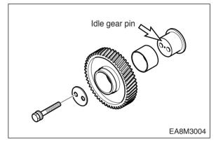
Install the idle gear by coinciding the marks impressed on the crank gear, cam gear, fuel injection pump drive gear, and idle gear.
