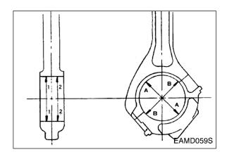
Compare the two values obtained through measurement of connecting rod bearing inside diameter with the outside diameters of crankshaft pins to determine the oil clearance.
