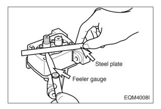
(2) With a feeler gauge, measure the amount of backlash between the oil pump drive gear and driven gear. Replace if the measured value is beyond the limit.
