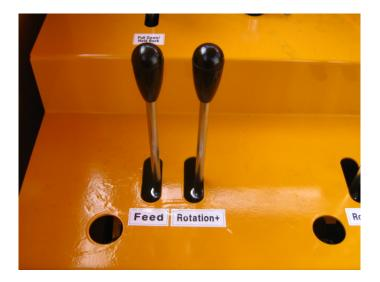
Feed : Fast up / down of the rotary head for rod changing. Rotation + : Rotary head rotation speed up.
