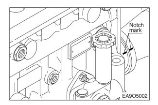
• Tighten the coupling fixing bolts and nuts to specified torque.
